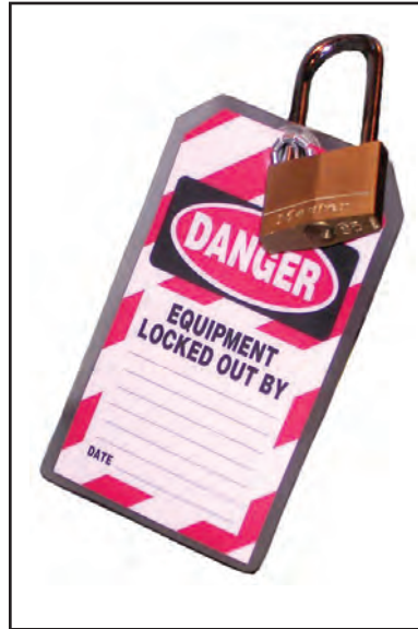
Figure 1-1: Example of a Lockout/Tagout Device
